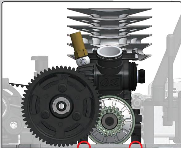
Adjust gear backlash by moving M3x8mm Flange Button Head Screw position.
