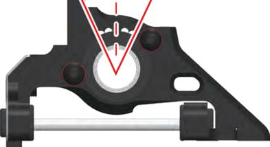
The belt will stretch and sag after a number of run. If the belt skips a tooth, adjust the belt tension one position tighter.
