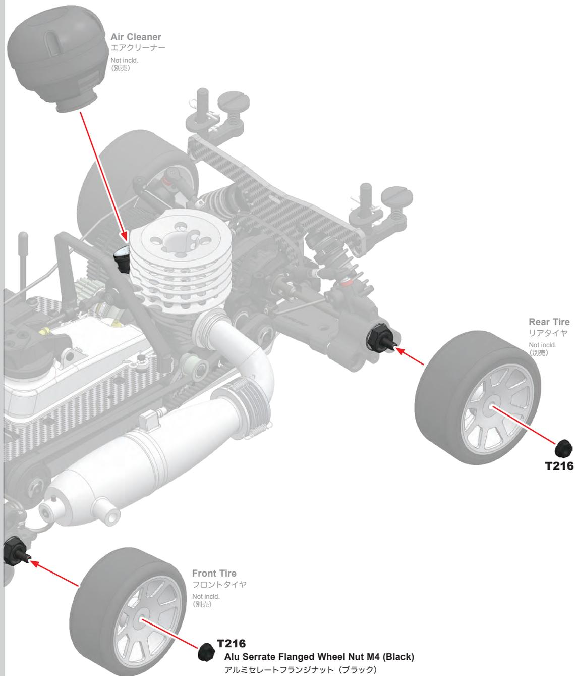
**Remove and retighten the nuts installed in the previous steps.**
