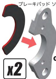
Apply epoxy adhesive to the black surface on the back to adhere.
