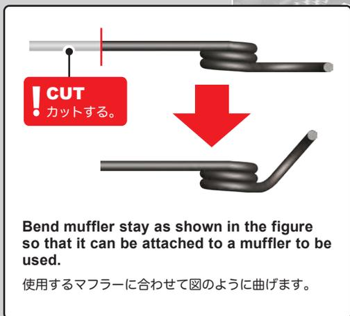
Bend muffer stay as shown in the figure so that it can be attached to a muffer to be used.
