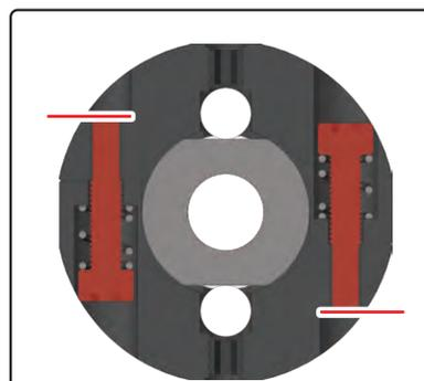
Tighten M2.6x12mm screw to align the tip of the screw with the notched surface of G015.
