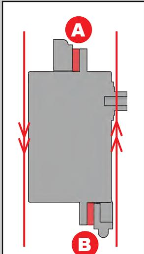
Adjust the thickness of the spacer (G012) to make the servo mount and servo parallel.
